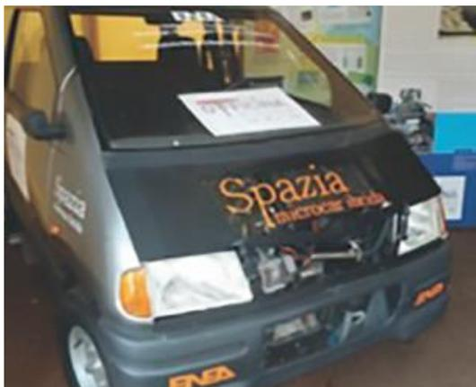
**ENEA HA PROGETTATO E RENDE DISPONIBILI PROTOTIPI DI VEICOLI DA CITTÀ ELETTRICI ED IBRIDI A ZERO EMISSIONI: URB-E, A TRAZIONE PURAMENTE ELETTRICA, E LA SPAZIA HPP (HYBRID POWER PACK), UNA MICROVETTURA CHE DIMOSTRA LA POSSIBILITÀ DI TRASFERIRE SU DI UN VEICOLO DI TAGLIA MINIMA IL CONCETTO DI IBRIDO “AUTOMOBILISTICO”, CON POWER-PACK TERMICO-ELETTRICO E BATTERIA DI PICCOLA TAGLIA (3 KWH).**
